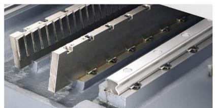
Equipped with patented in-house linear motor featuring with high responsive, zero vibration, zero backlash, long life, zero maintenance to provide excellent working accuracy.
