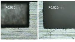
Workpiece Material: SKH9 66 ■ Electrode Material: Copper Mirror Finish 1 Processing Depth: 1.275mm Roughing Time: 14 min 20 sec Fine Finishing Time: 2 hr 37 min
