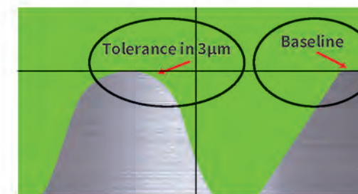
Linear motor models (Radius tolerance in 3μm) Magnification: 120x
