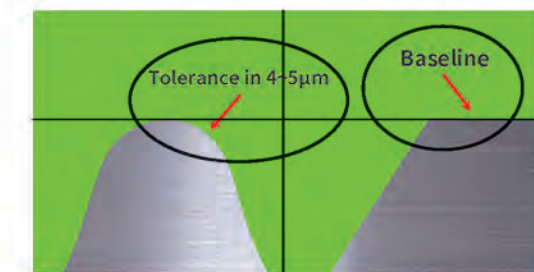
Conventional Ballscrew models (Radius tolerance in 4~5μm) Magnification: 120x
