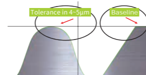
Conventional Ballscrew models (Radius tolerance in 4~5µm) Magnification: 120x
