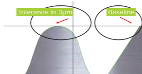
Linear motor models (Radius tolerance in 3µm) Magnification: 120x
